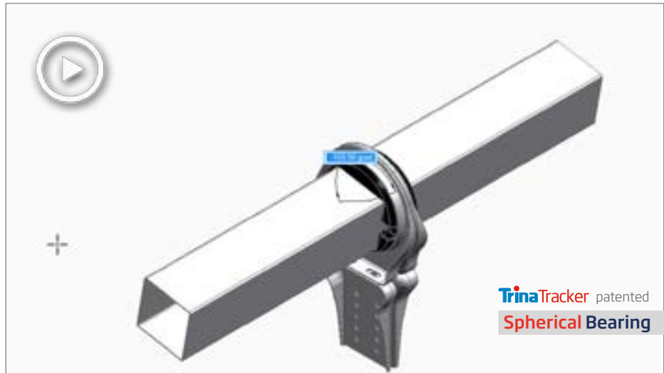
Video 2: Spherical bearing rotation
