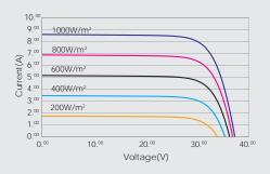
Average efficiency reduction of 4.5% at 200W/m $^{2}$  according to EN 60904-1.
