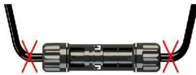
Wrong way for the cable
