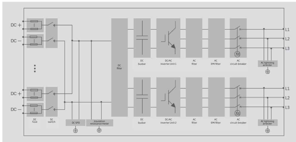
Figure 17 - Schematic of the central inverter supplied by Manufacturer S
