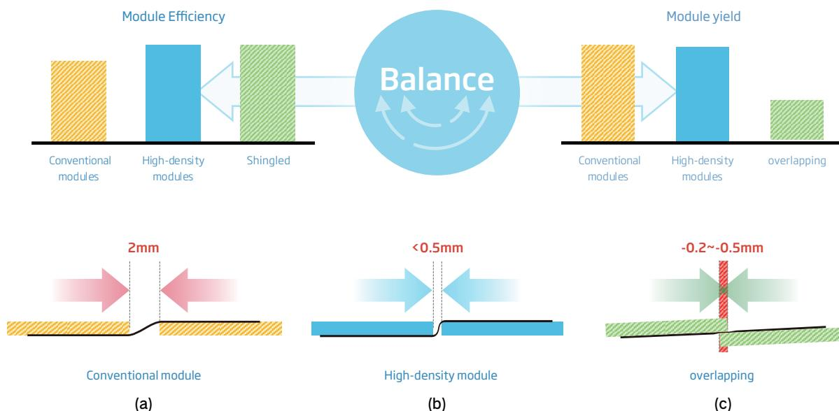
Figure 10 - Conventional Module vs. High-density cell interconnect Module
