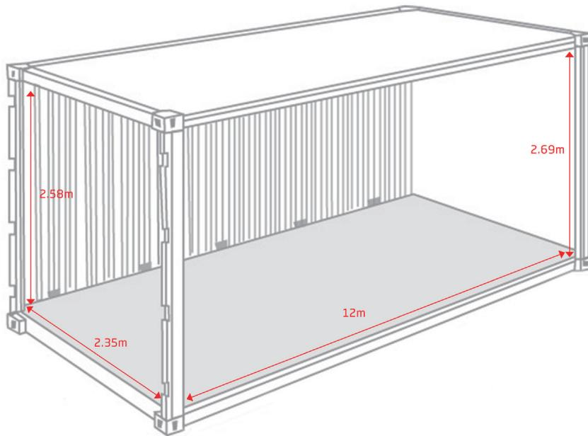
Figure 14 - Common 40 HC container dimension
