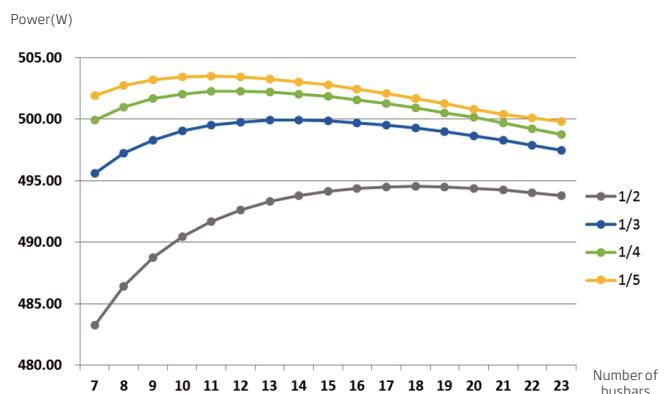
Figure 7 - Power simulation concerning different cutting options and busbar numbers
