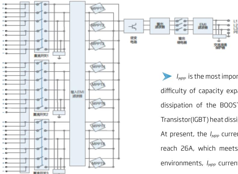
Figure 18 - The electric circuit of the string inverter of H manufacturer
