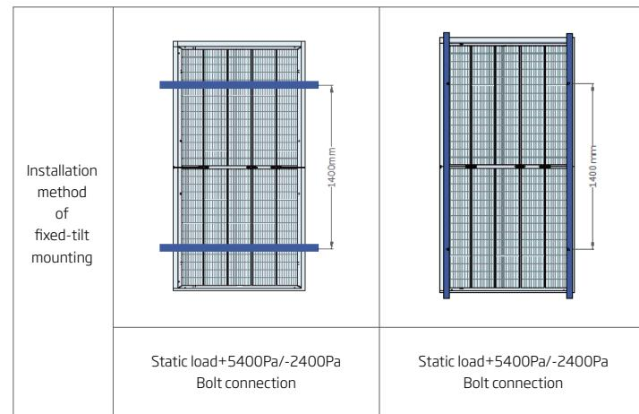
Figure-19 Matching the installation positions for fixed-tilt mounting
