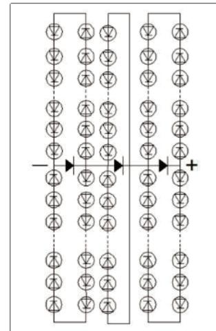
Figure 8 - Circuit configuration of the Vertex module and distribution of the bypass diodes
