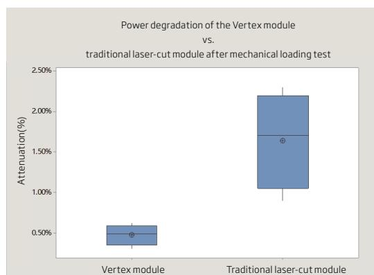
Figure 12 - The Vertex backsheets Module vs. Typical Laser-cut backsheets Module: Power degradation
