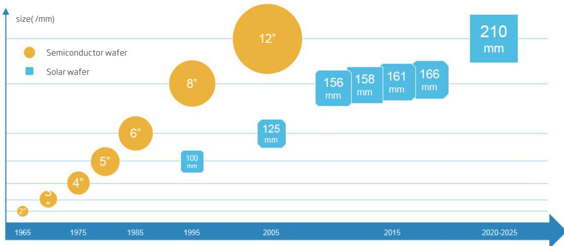
Figure 5 - Development in the semiconductor and the solar wafer sizes
