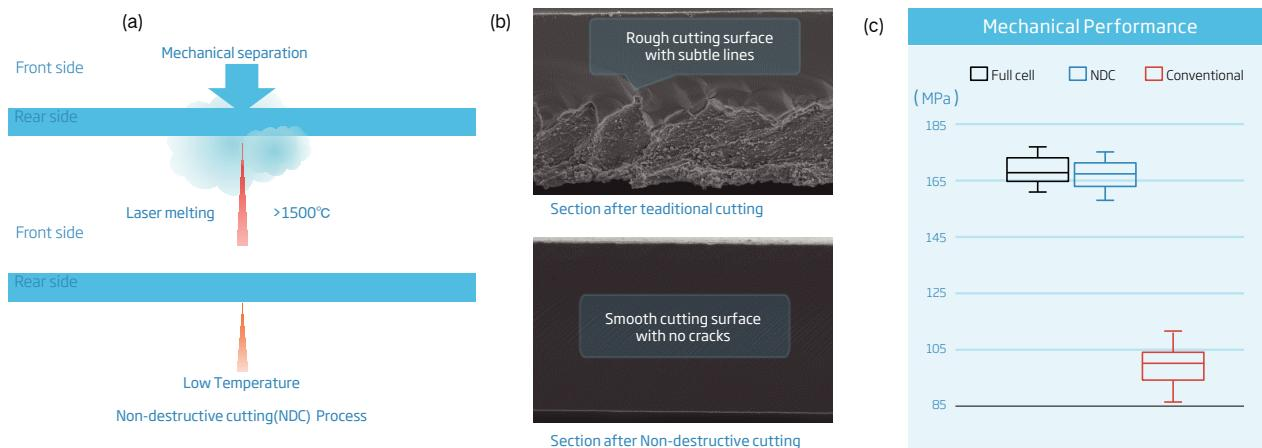
Figure 9 - Traditional Cutting vs. Non-destructive Cutting: (a) Cutting process;
