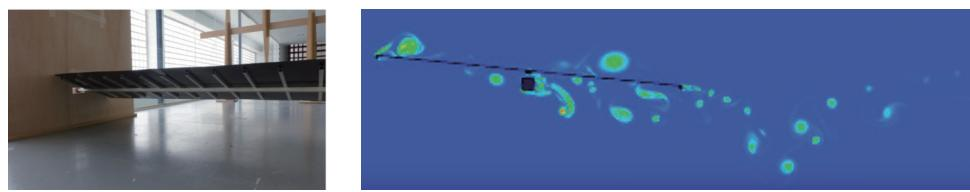
Figure-23 Simulation of resonance and flutter of the tracker matching the Vertex module
